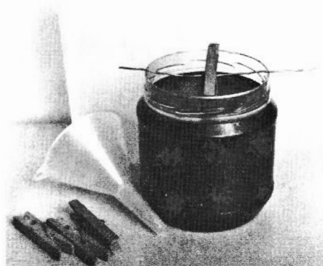
Fig. 4: The G3RJV etching assembly! Clothes pegs (once used for this job, don't even consider them for wash-day ever again!) provide a simple and secure way of holding the p.c.b. vertically in the etching fluid (see text).
